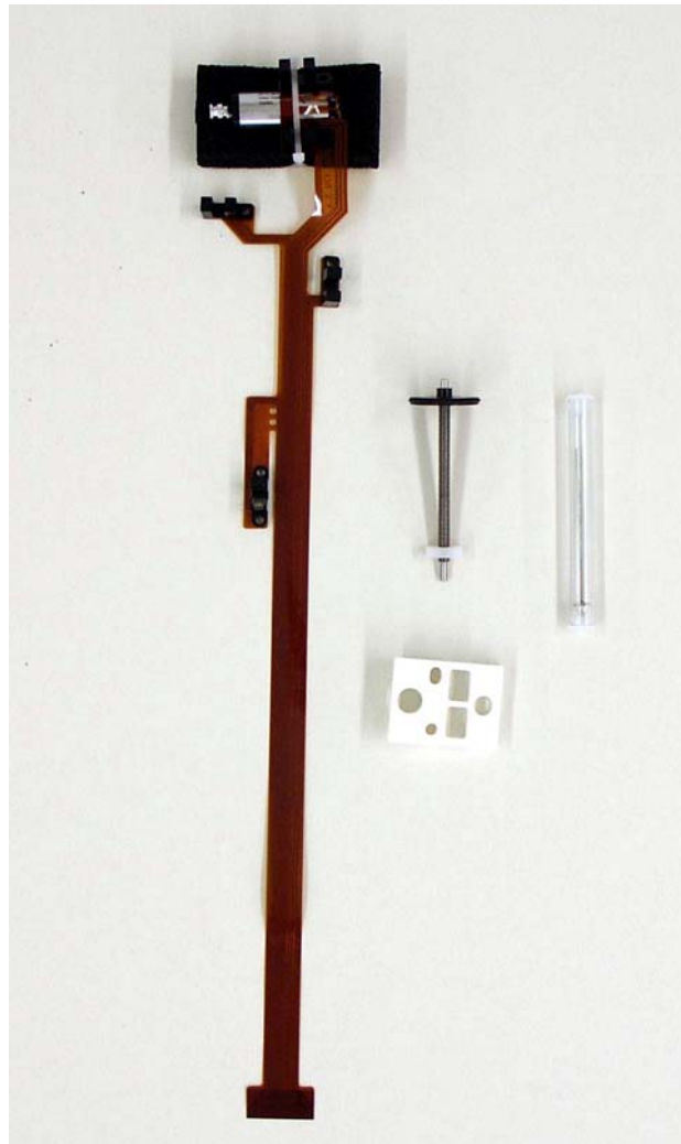
Figure 2. Contents of needle unit repair kit. Left: Flex print with motor. Middle (top): spindle assy. Middle (bottom): needle unit body. Right: pre-puncturing needle.
